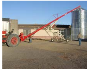
PTO-powered grain auger loading pellets into storage silo.
