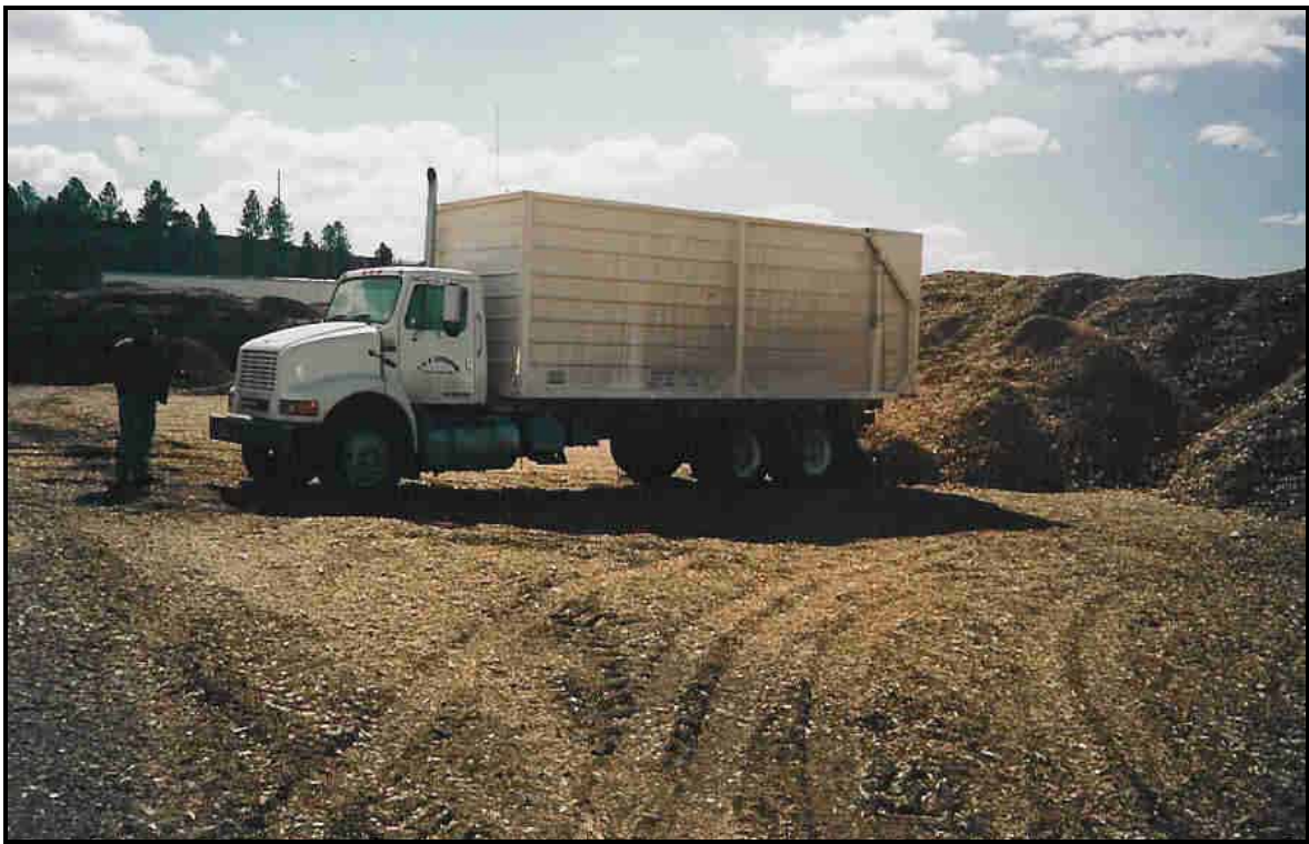
Photo 4: Trucks unload either at the heating plant or the open storage pile depending upon need. CSC tries to maintain piles at about 1,000 tons. In the picture pile is estimated at 800 tons. Chips are used within a year.
