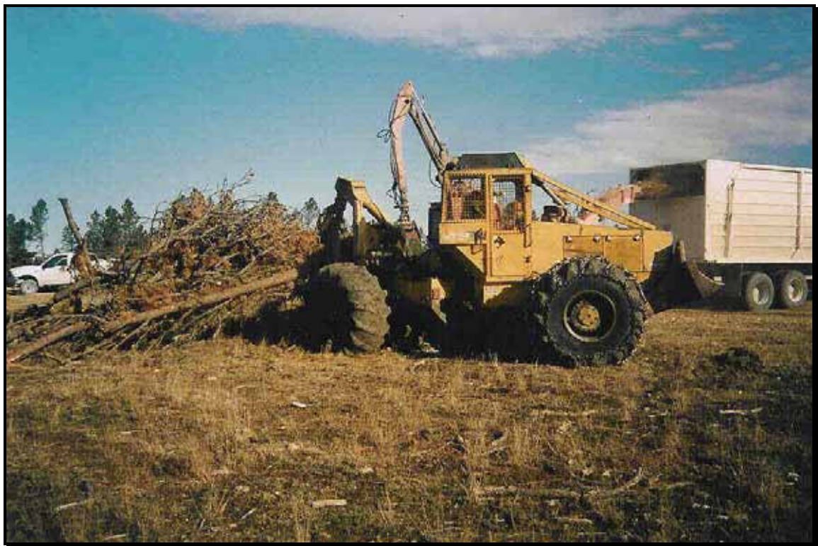
Photo 8: Skidder positioning slash within reach of chipper's grapple.
