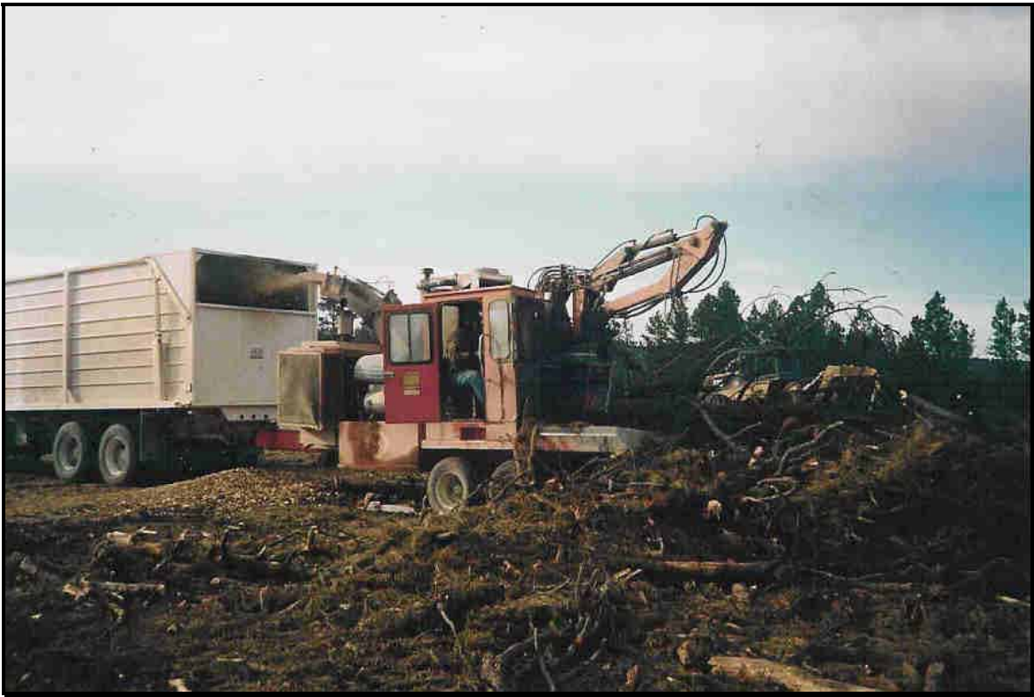
Photo 6: Chipper is hitched to truck with pintle hitch for stability and blows load directly into the truck. In good conditions it takes about 20 minutes to load 10 tons.
