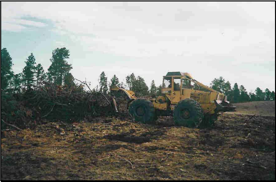
Photo 7: Chipper cannot work directly out of slash piles as it would necessitate constantly moving the unit. Chipper is fed by a log skidder with hydraulic grapple to optimum production.
