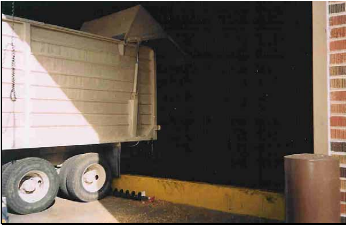
Photo 2: Truck with live floor unloading 10 tons into below-grade storage bin.
