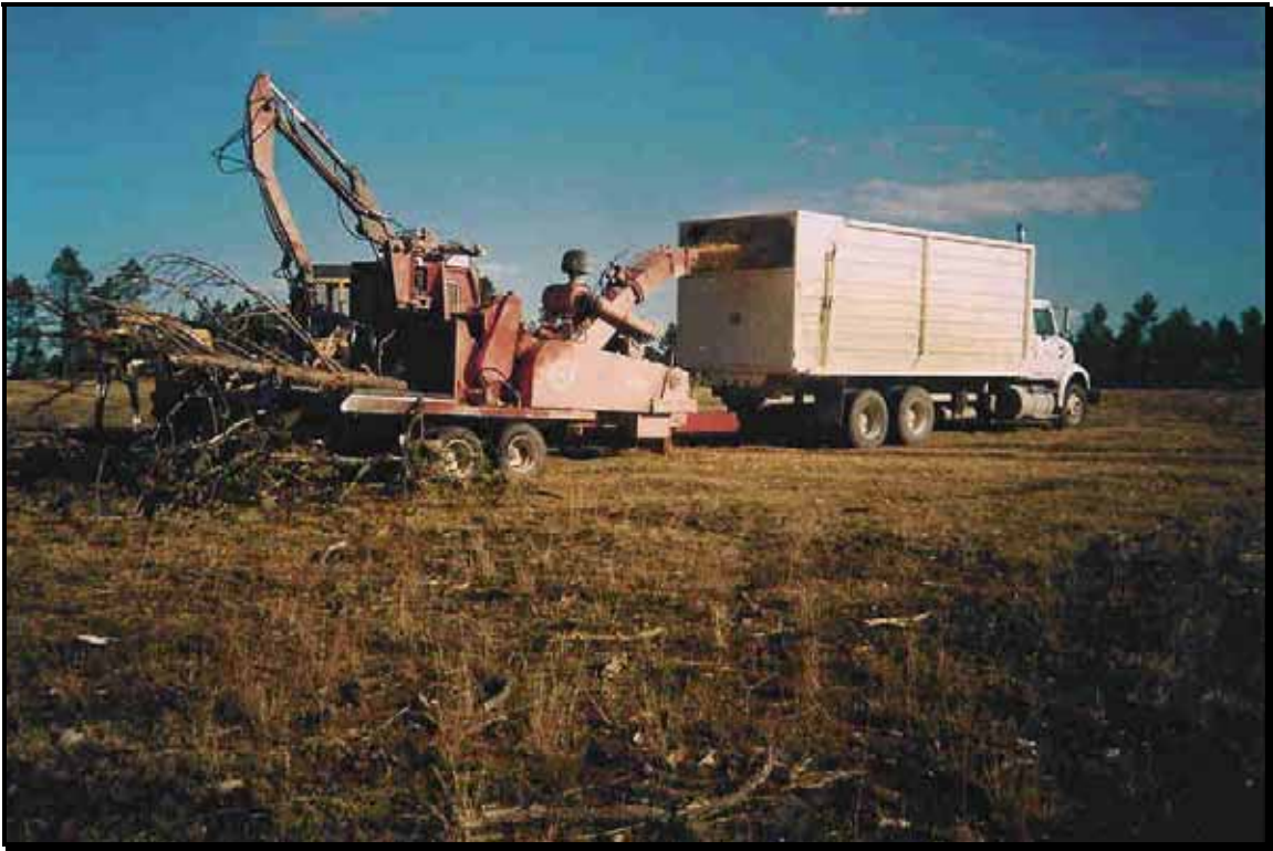
Photo 5: In the woods the chipper is a Morbark 30-36 with a 330 horsepower Caterpillar engine, considered near optimum for the operation.
